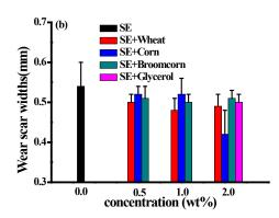
**Figure 1:** average COFs (a) and wear scar widths (b) for the lubricants for steel-aluminum pair at different additive concentration at 20 N, 5 Hz and RT
