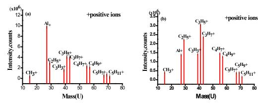
**Figure 6:** TOF-SIMS spectra of positive ions in the worn surfaces lubricated by (a) neat SE base oil and (b) SE with wheat leaf-surface wax at room temperature
