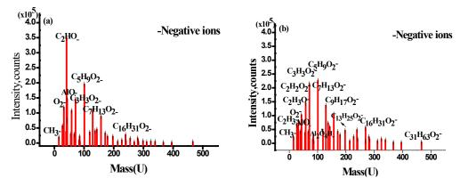
**Figure 7:** TOF-SIMS spectra of negative ions in the worn surfaces lubricated by (a)neat SE base oil and (b)SE with wheat leaf-surface wax at room temperature
