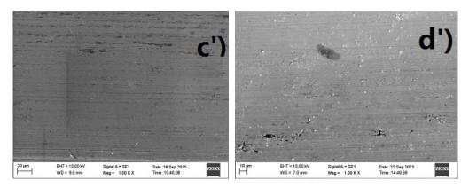
**Figure 5:** SEM images of the worn surfaces lubricated by (a') SE base oil, (b') broomcorn, (c') corn, and (d') wheat
