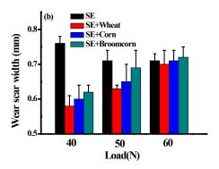
**Figure 4:** average COFs (a) and wear scar widths (b) for the lubricants for steel-copper pair at different loads at 5 Hz and RT
